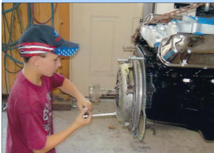
Cameron (above) and Sidney (below) installing the clutch assembly and fly wheel
