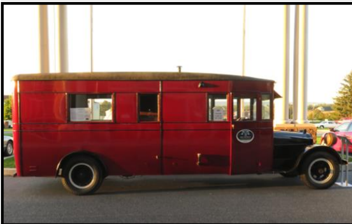
1917 Packard motorhome with 424-ci, twin-six V-12 engine
