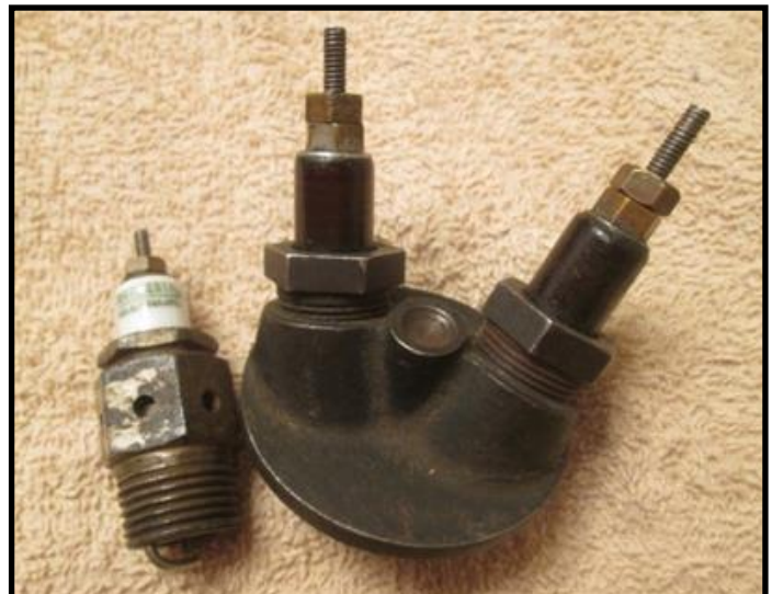
Circa 1903 single cylinder Cadillac spark plug
