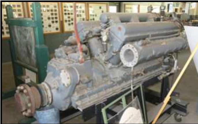
Packard 4M 2500 12-cylinder, 2,490-ci PT boat engine
