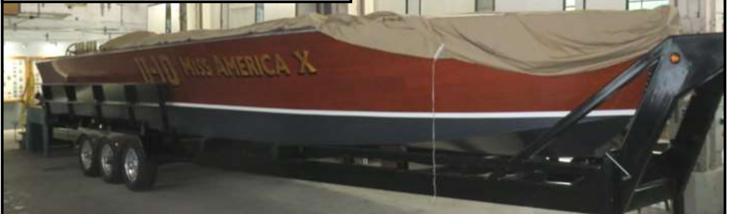
The 1932 Garfield "Gar" Wood "Miss America X"—the last powerboat built by Gar Wood and the only one built with four Packard V-12 engines, each producing 1,800 horsepower. In 1932 it set the world water speed record of 125 mph—a record that held until the mid-1960s
