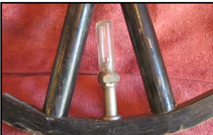
An unusual valve stem leak detector displayed on a section of an antique wood spoked wheel.
