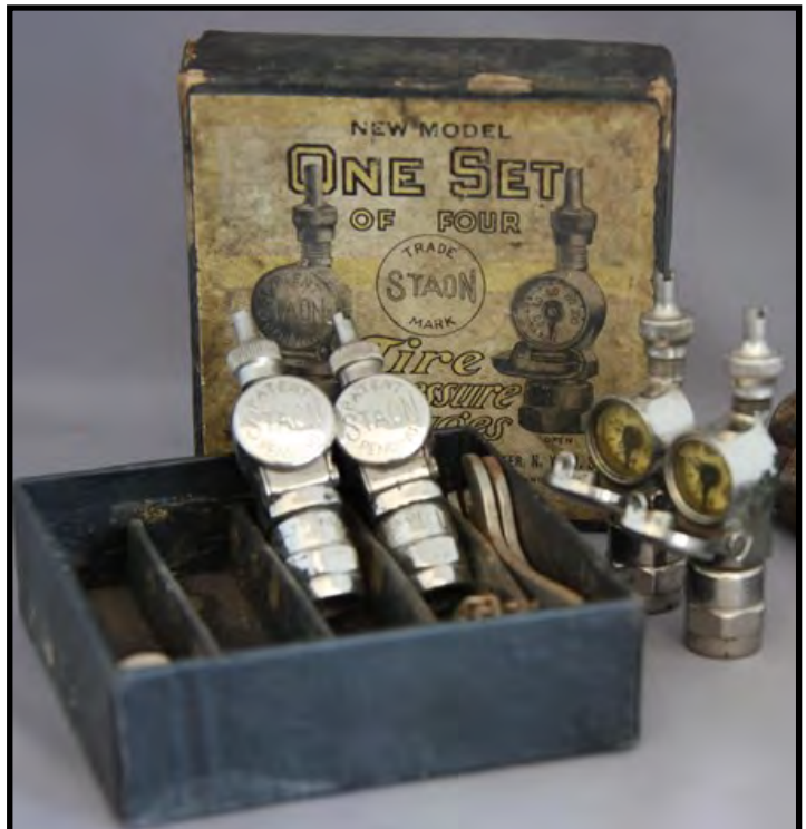
This boxed set of four unique valve stems has a built-in pressure gauge. Unfortunately, I did not bid high enough to add this great set to my collection of tire related artifacts.
