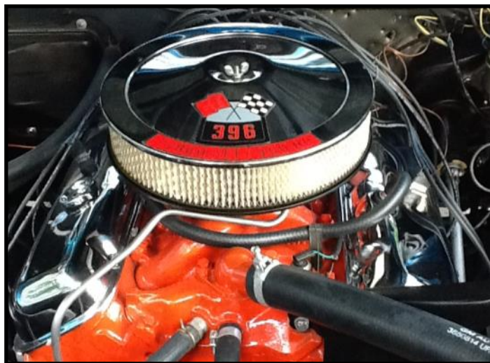
Rebuilt L-34 396-ci, 360-hp engine in Bob's 1966 Chevelle SS-396
