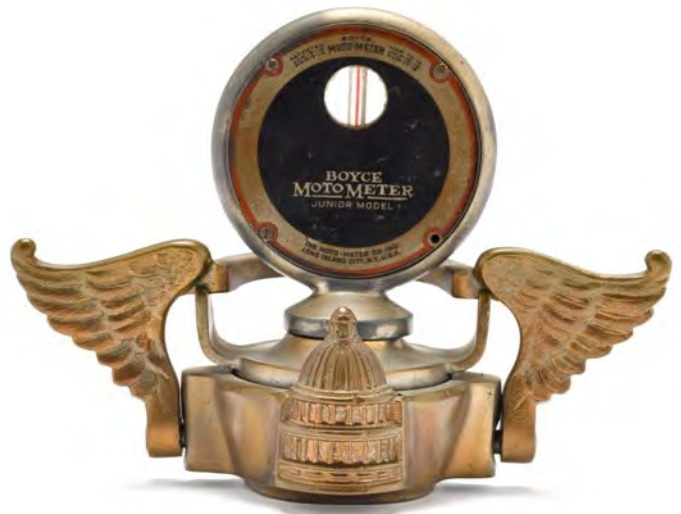
This radiator cap holds a Boyce Motometer (temperature gauge) and has an image of the US Capital on front. That part is actually a latch that when pressed releases the top of the cap so water can be added without unscrewing the entire unit.
