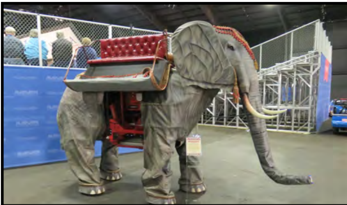
Wendell the Elephant—built in 1951 and restored in 2013-2014. Powered by 4-cylinder engine & has 2 forward & 1 reverse speeds.
