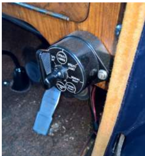
The driver's control for the Wilcot signals. Distracted driving at its best.
