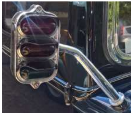
Wilcot traffic signal installed on a 1933 Morris Isis.
