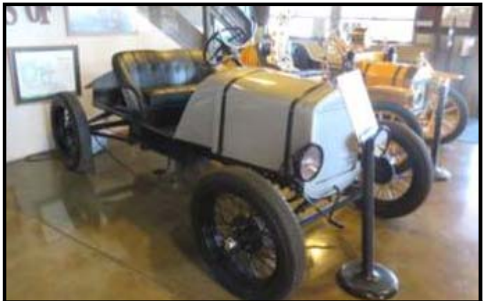
1910 Ford Model T, which was converted into an electric car
