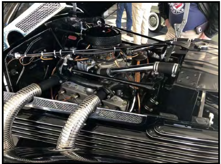
The engine bay of the Cord, showing off the supercharger.
