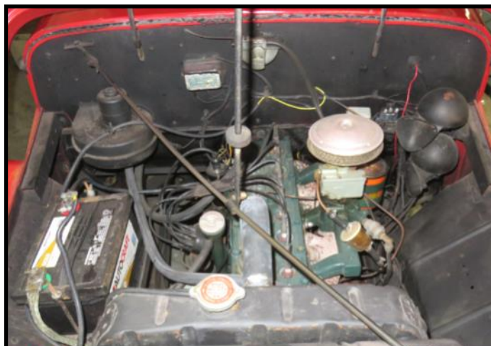
The Jeepster's powerhouse 161-cid, 6-cylinder engine
