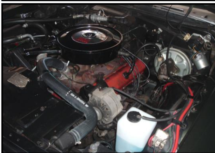
Close-up of the Delta 88's original, unrestored 455-ci engine
