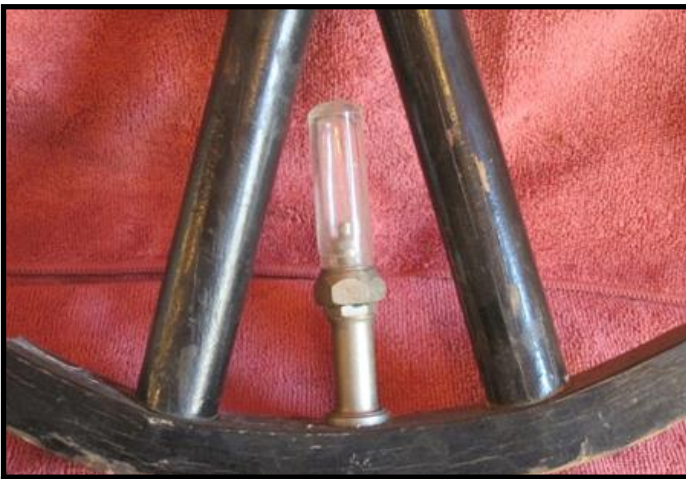
Glass air leak warning device for tire tube valve stems
