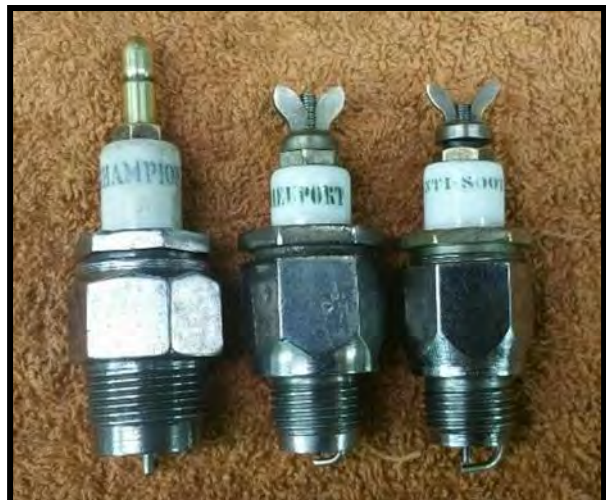
Left – one of the early plugs produced by Albert Champion after he left the Stranahan's. Center - Neuiport spark plug imported from France, produced by Champion. Right is a similar style of plug made in France for the American market, branded "Anti-Soot" French clay insulators were superior in quality and were used in many early plugs.
