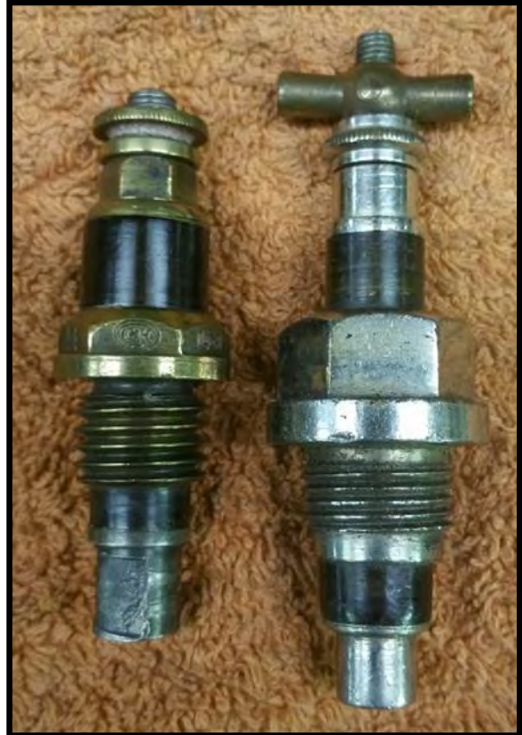
Two pre-1900 make-and-break ignitors.
