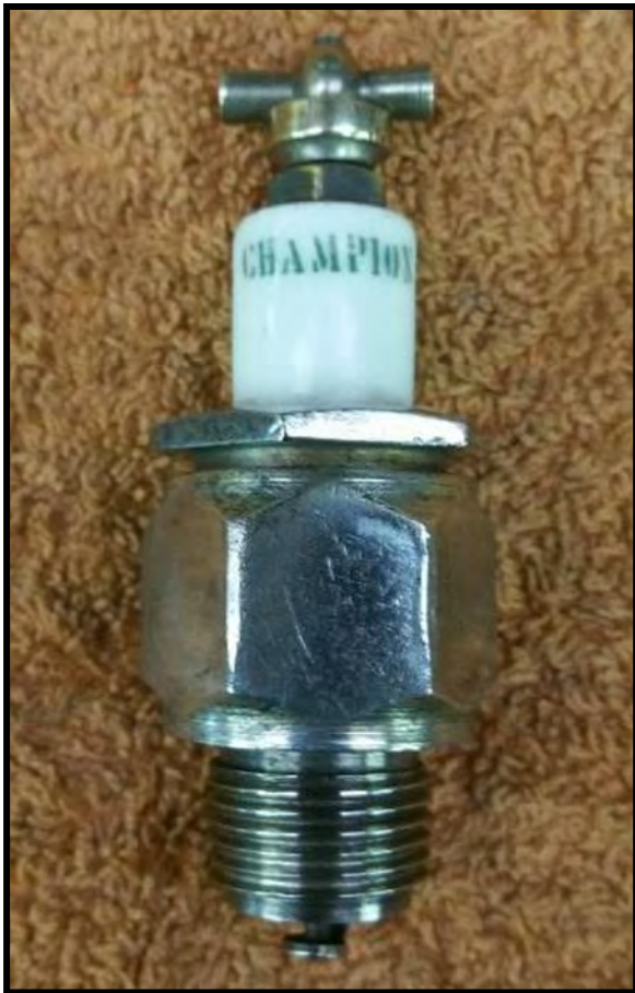
An example of the first plug manufactured with the Champion name printed on it. Note the similarity to the Neiuport spark plug shown above.
