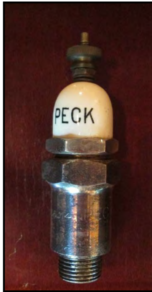
Peck adjustable gap spark plug made in Scotland
