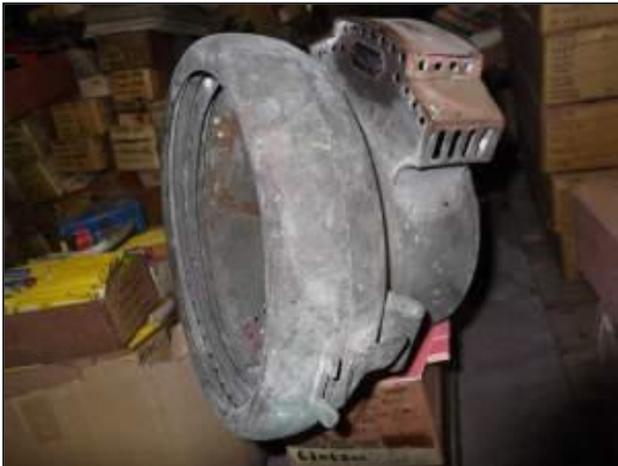
A rare but badly corroded French headlamp
