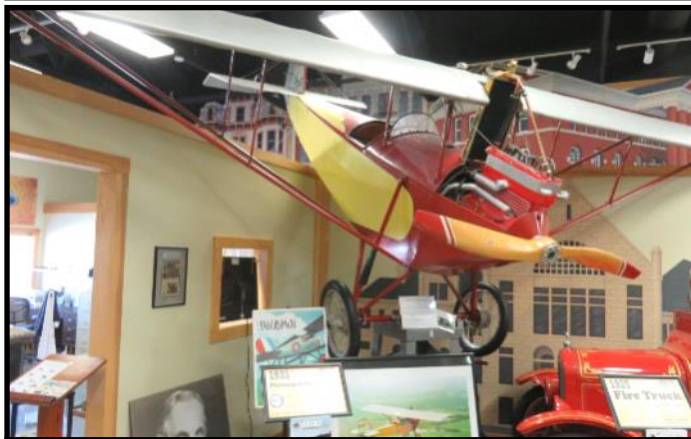
1931 Pietenpol Sky Scout airplane with a Model T engine
