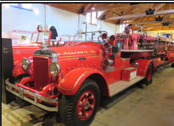
1935 Mack Ladder Truck—75-ft wooden aerial ladder
