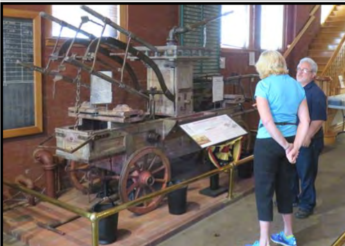
1792 hand-pumper—probably the oldest in original, unrestored condition in the United States—could pump 150 gallons/minute
