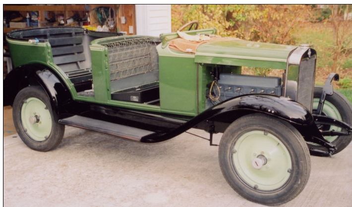
After painting, the process of reinstalling body parts began. Getting the center door posts on correctly was the biggest challenge.
