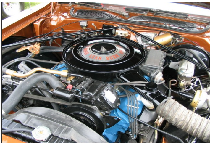
Lean Burn System, computer and vacuum advance is to the right of the air cleaner
