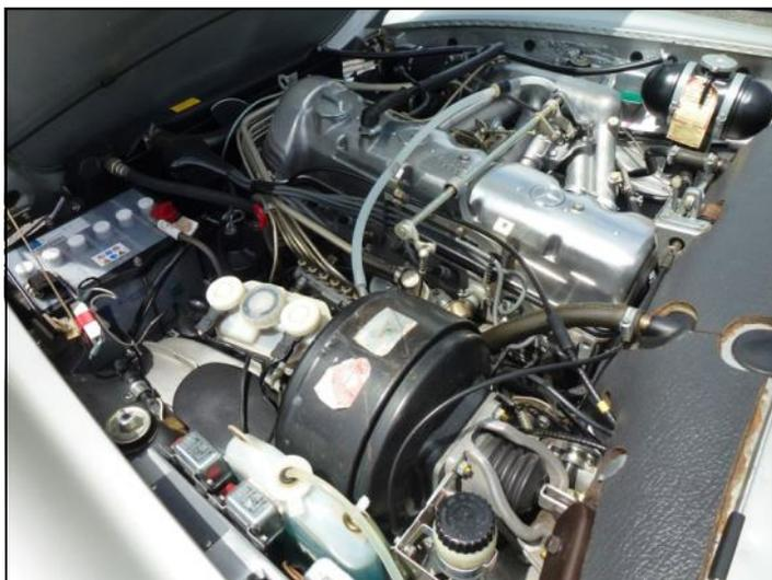
*The 2778cc 6-cylinder engine produces 170 horsepower. Each engine was bench-tested for two hours before being fitted.*
