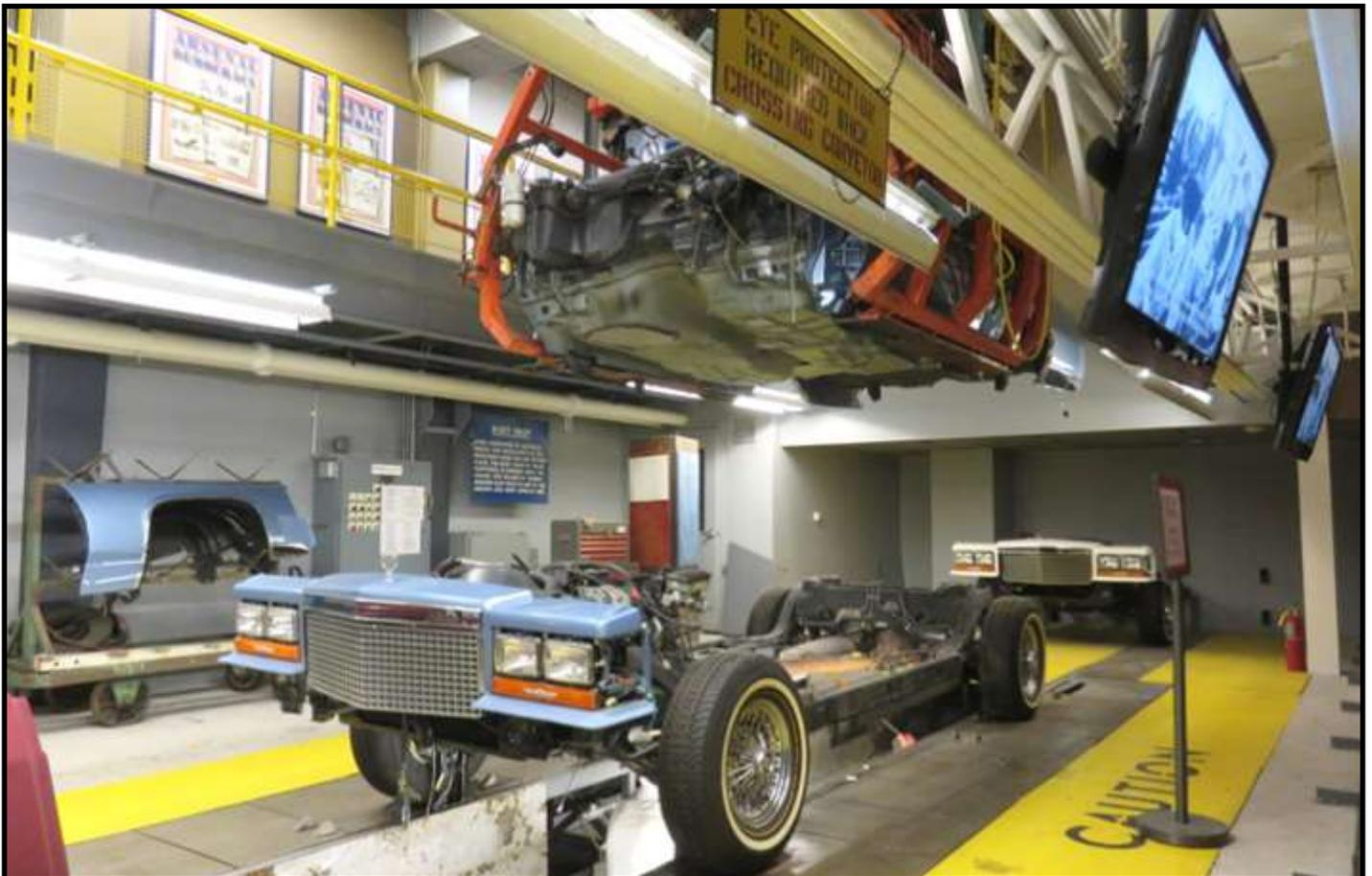
*"Body drop" assembly line—this portion was removed from the Cadillac Clark Street Assembly Plant which operated from the 1950s until 1987*
