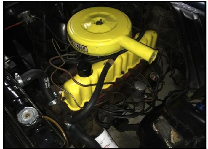
*The Comet's original 260-cubic inch straight six-cylinder engine*
