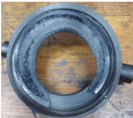
Badly worn throw-out bearing. Note the missing chunk at the bottom.
