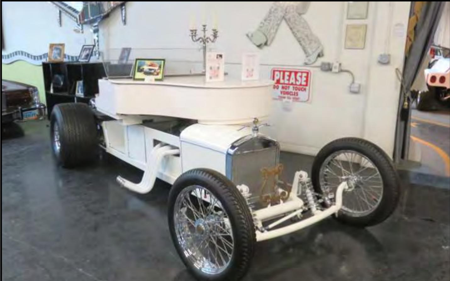
*The “Piano Car”—the world's fastest piano—a 7-ft Schaefer & Sons grand piano mounted on a tube frame with a 350-ci V8 engine*
