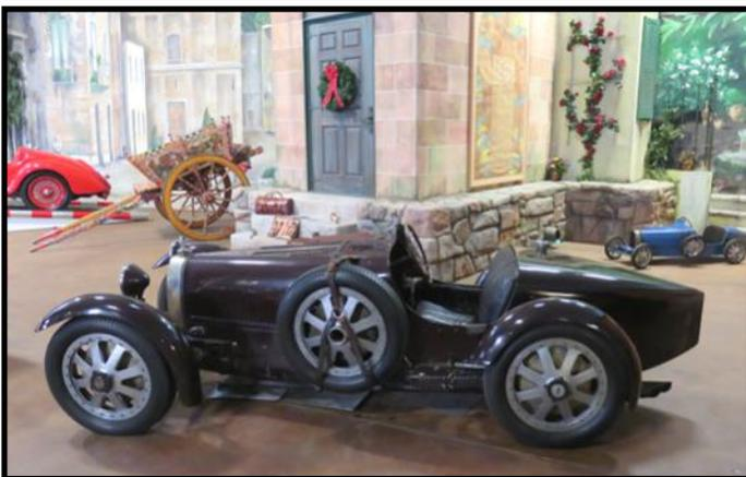
*1926 Bugatti Type 35 with 1.99-liter, inline 8-cyl, 95-hp engine*
