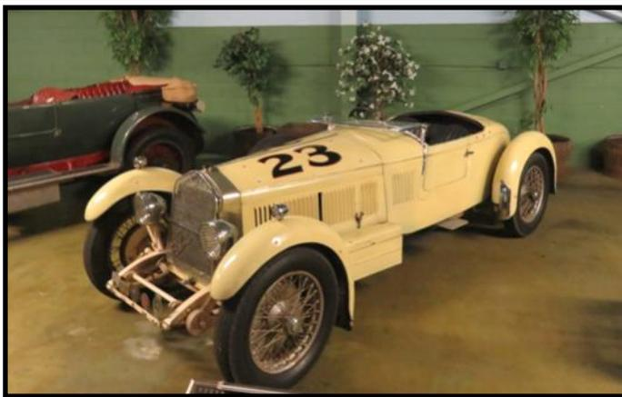
*1929 Alfa Romeo 6C with supercharged inline 6-cyl, 85-hp engine*
