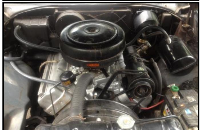
*The 1956 DeSoto Fireflight has a 330-ci, 230-hp V-8 hemi engine*
