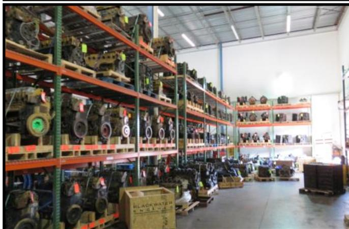
*Diesel engines in line to be remanufactured at Blackwater Engines*
