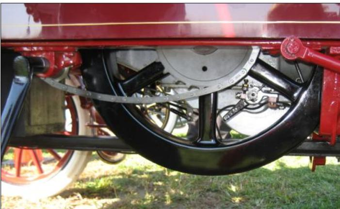
*No starter motor— it took brute strength to spin the crank which is connected by chain to the huge flywheel of the single cylinder engine. This really is a get-out-and-get-under car.*
