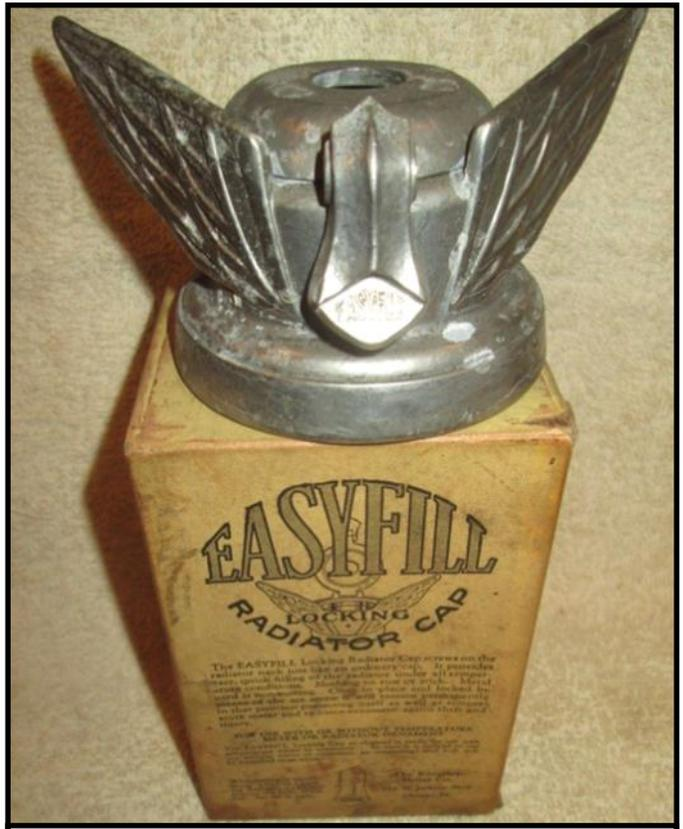
NOS "Easyfill" radiator cap designed for a MotoMeter
