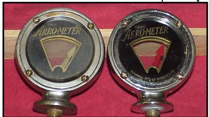
*Front and back of Aero-Meter radiator temperature gauge*
